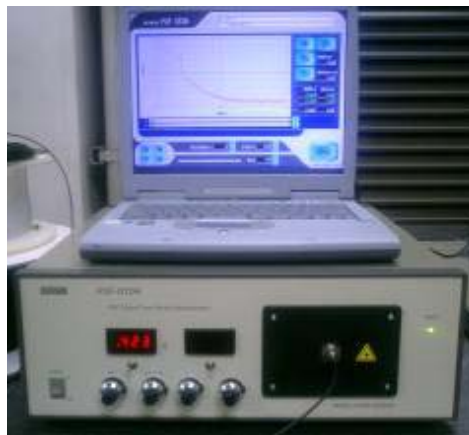
Fig. 2 Photo of the instrument, OTDR-2000, Scientex inc., used in the experiments.
