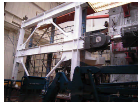
Full-scale brace test
