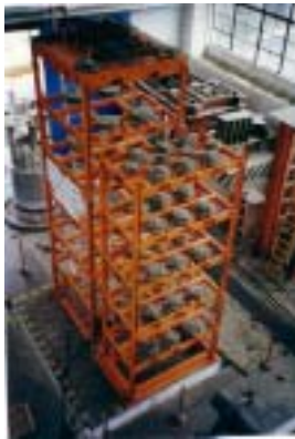
Figure8 Adjacent Structure Linked by Fluid Dampers
