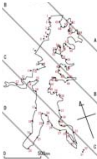
Fig. 8 Observation points along the reservoir for the ground survey
