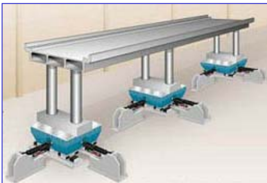
Fig. 2 Shared Use Shaking Platforms, Univ of Nevada, Reno
