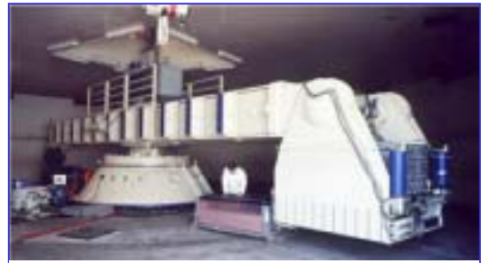
Fig. 5 Shared Use Geotechnical Centrifuge, UC Davis
