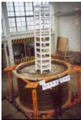
Figure22 Shaking Table Tests on SSI model
