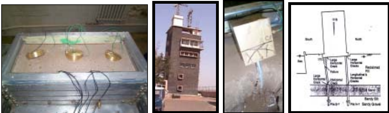
Figure 6: Model test and field case history; (a): Pile foundation after the dynamic centrifuge test; (b): Failed Kandla Port tower; (c): Hinge formation in the centrifuge test; (d): Hinge formation in a building, Tokimatsu et al (1997).
