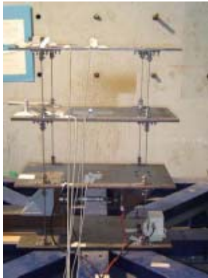
Fig. 7 Setup of shaking table test
