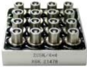
Figure 1 Planar Pitch-Catch Array Probe
