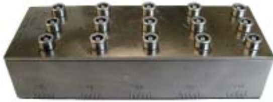
Figure 5 Planar Tandem Array Probe
