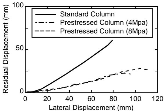
Fig. 7 Effect of Prestressing on the Residual Displacement of Unloaded Columns [Ikeda 1998, Ikeda et al 1998]
