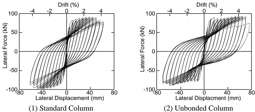
Fig. 4 Lateral Force vs. Lateral Displacement Hystereses
