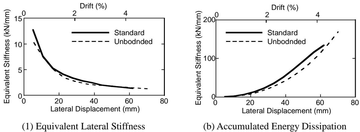
Fig. 5 Equivalent Lateral Stiffness and Energy Dissipation
