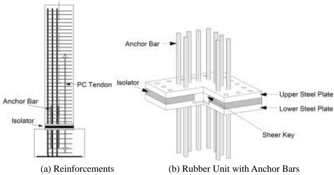
(a) Reinforcements (b) Rubber Unit with Anchor Bars
