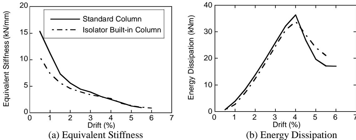
Fig. 13 Effect of Isolator on the Equivalent Stiffness and Energy Dissipation
