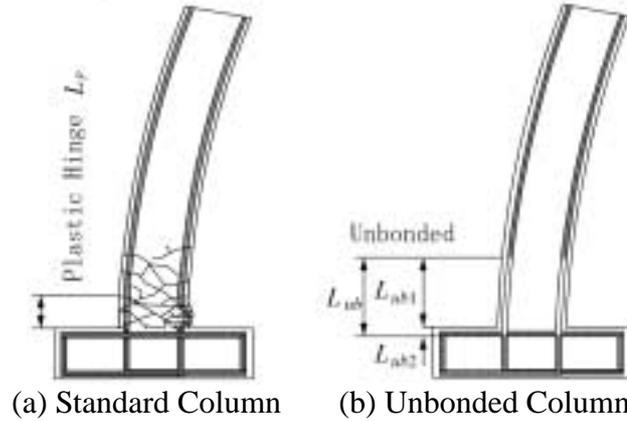
Fig. 2 Unbonding of Longitudinal Bars
