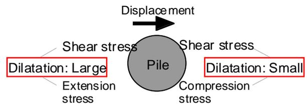
Fig. 9 Stress states around pile
