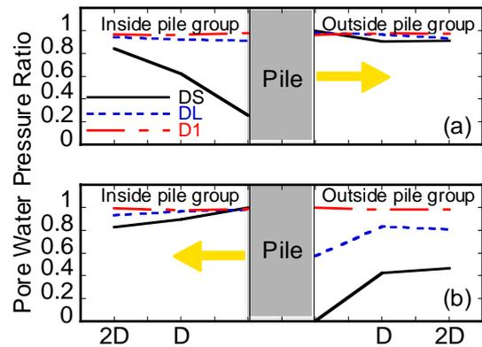
Fig. 15 Reduction in pore pressure around pile in DS, DL and D1
