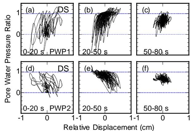
Fig. 8 Relationship between relative displacement and pore pressure ratio in DS
