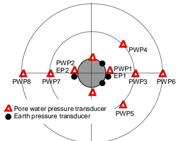
Fig. 2 Instrument on and around pile
