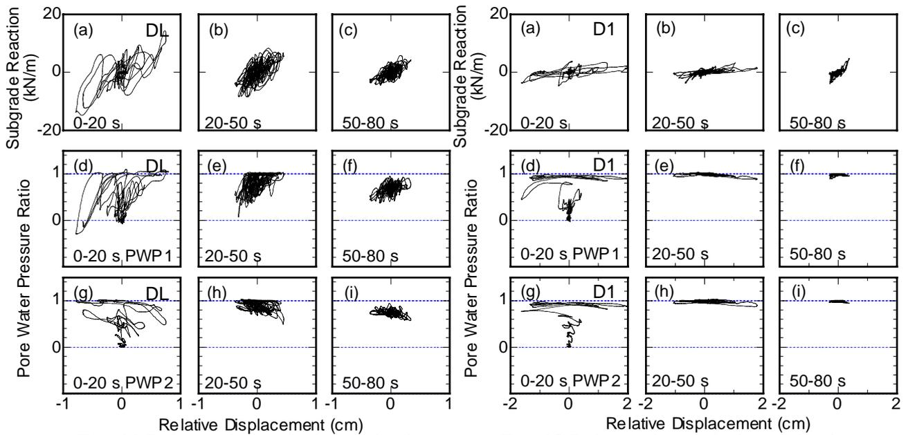
Fig. 11 Relationships of relative displacement with subgrade reaction or pore pressure ratio in DL
