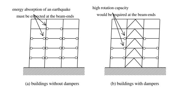
Fig.2 a seismic design based on damage at the beam-ends (low-rise or medium-rise buildings)
