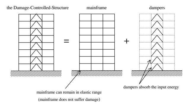
Fig.1 the Damage-Controlled-Structure (Wada et al., 1992 and Y. H. Huang, 1995)
