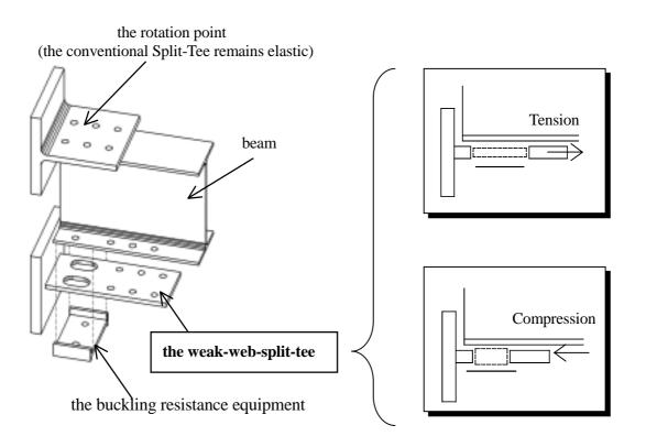
(a) detail of beam-to-column connections
