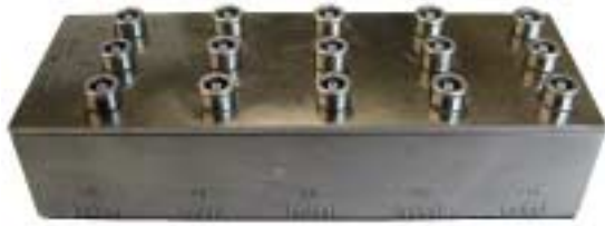
Figure 5 Planar Tandem Array Probe
