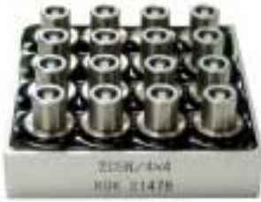
Figure 1 Planar Pitch-Catch Array Probe
