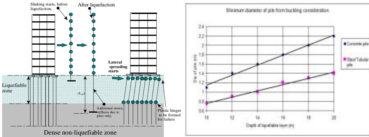
Figure 7: (a) Possible failure modes of pile foundation in a liquefiable region; (b): A proposed minimum pile diameter requirement to avoid buckling, details can be seen in Bhattacharya (2003).
