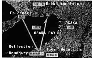
Fig.11 Concept to explain a possibility of long-period later phase in Fig.10 with surface waves across the Osaka bay.
