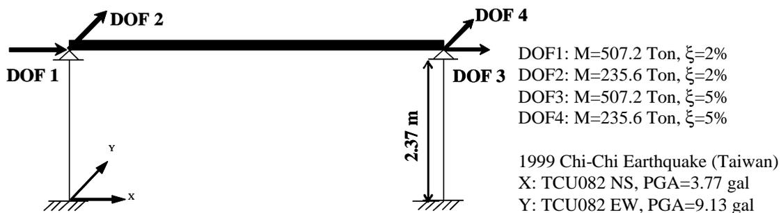
Figure 18 Pseudo-dynamic DSCFT Tests using Application Protocol Approach
