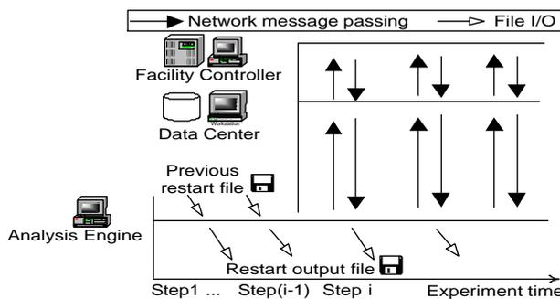
Figure 12b A restart experiment completing a previously disconnected experiment
