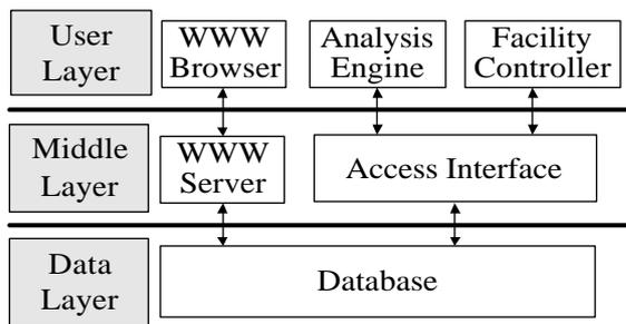
Figure 11 Three-layer framework of the Database Approach
