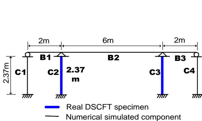
Figure 15 Substructure Pseudo-dynamic DSCFT Tests using Database Approach
