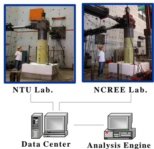
Figure 16 Configuration of the DSCFT Tests using Database Approach
