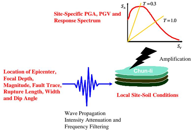
Figure 2. Procedures in estimation of ground motion intensities.
