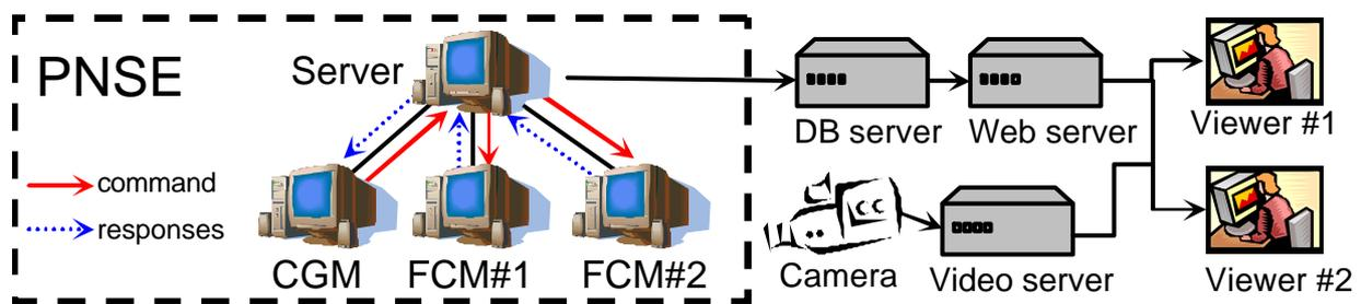
Figure 14 The Architecture of the Application Protocol Approach
