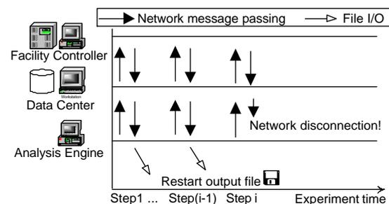
Figure 12a Experiment encountering an accident network disconnection
