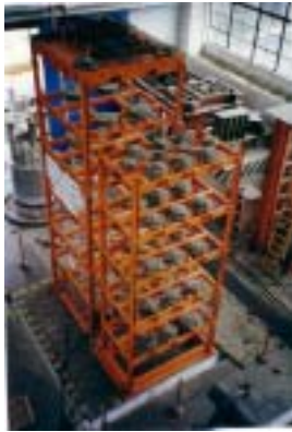
Figure8 Adjacent Structure Linked by Fluid Dampers
