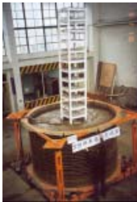
Figure22 Shaking Table Tests on SSI model
