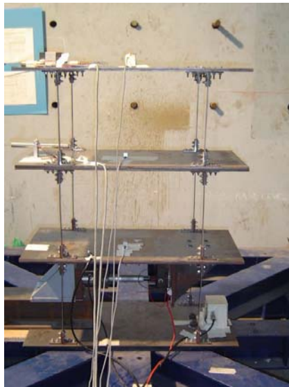
Fig. 7 Setup of shaking table test
